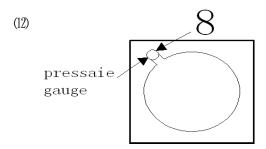
Pressure will now build up in the pot. The normal running pressure is 8 psi.
