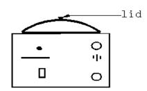
Replace the lid ensuring it is fitted squarely and tighten the 1c knob 2full turns of the lid knob should be enough.
