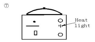
When the oil has reached the correct temperature the amber heat lamp will go out.
