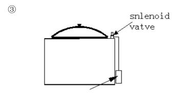
Place is small container under the outlet pipe at the back of the machine to catch any steam and water expelled when cooking finishes.
