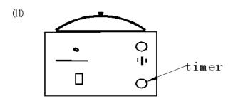
Set the timer on the front panel to the required time. You may hear a click as the sciaenid valve closes.
