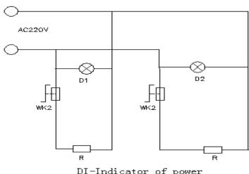
DI-Indicator of power WK2-Temperature controller R-Heat tube
